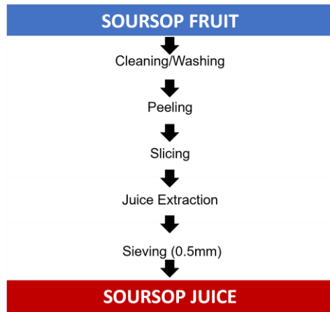
Fig 1: Process flow chart for soursop juice production Source: Ogodo et al., (2015)
