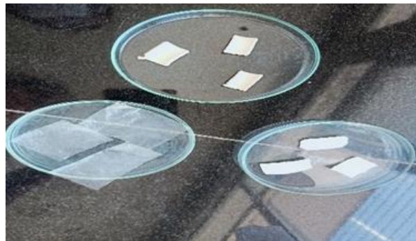
Fig 3: Top-to-bottom: First row- PVC plastic strips; Second row (Left-to-right)- LDPE plastic strips, HDPE plastic strips
