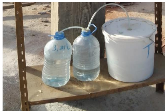
Fig 5: The digester used.
